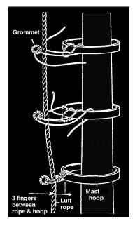
In a traditional method of bending the sail to the mast (left), mast hoops are seized to grommets on the sail's luff. Using light marline, a tag hitch is taken around the hoop, and the free ends passed through the grommet (top). The ends are then passed back through the hoop (center), and several turns taken around all parts (bottom). The seizing must be just slack enough so the hoops lie at right angles to the luff rope.
