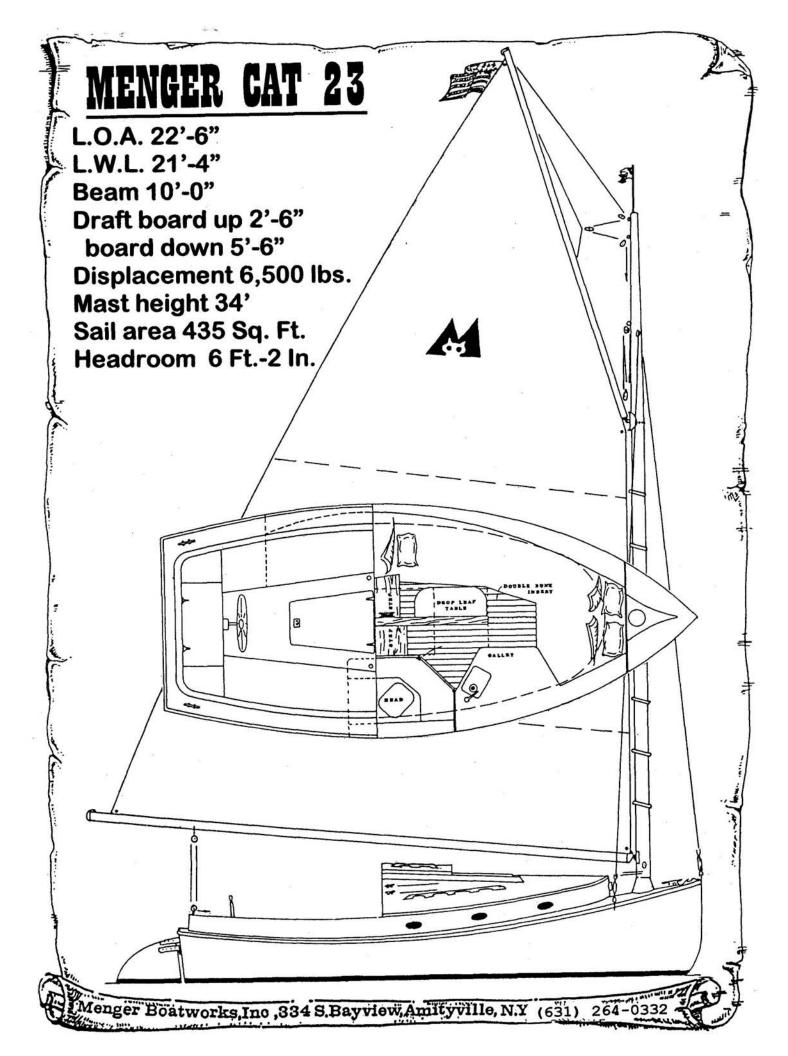
The Menger Cat 23 is a variation of a 1935 Sweisguth catboat design. The under water shape and sail plan are the same. This design is renowned as being the fastest of the 20'-25' Cats. We have made numerous design enhancements to the deck and interior arrangements to allow for more comfortable and functional living arrangements.
